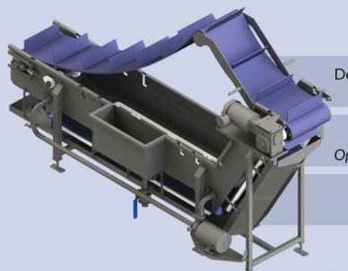
Designed to allow belt to run in the cleaning position, to aid in proper sanitation
